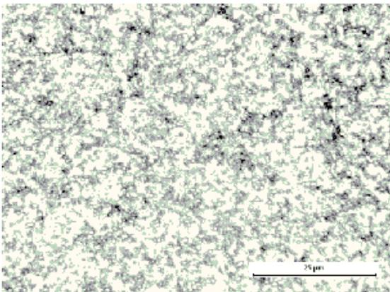
Figure 2. Sandvik 13C26 hardened and tempered.
